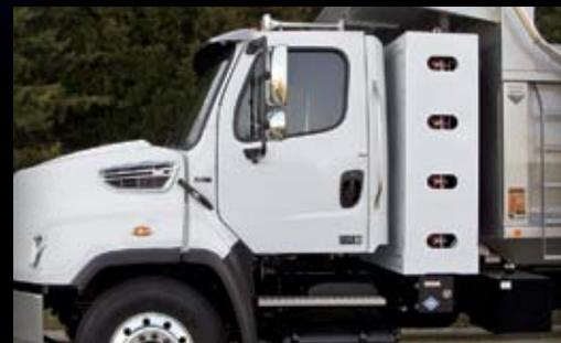
CNG tanks mounted back-of-cab.
